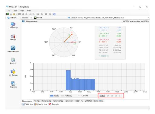
Online measurements in graphical form – phase diagram and daily total active power consumption histogram
