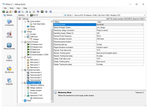
Settings for power quality parameters are set with setting and monitoring software MiQen
