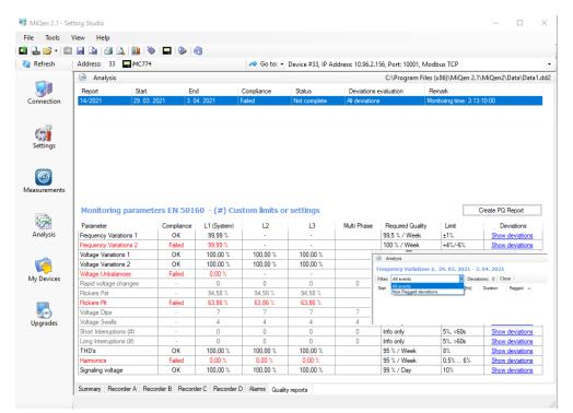
By clicking on "Show details" for each PQ parameter MiQen displays time-stamped measurements (events), which were outside limit lines
