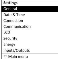
General settings are essential for *iMC7×0 Power Monitoring Device*. They are divided into four additional sublevels (Connection, Communication, Display and Security).
