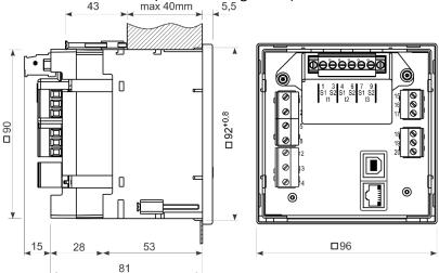
Dimensional drawing and rear connection terminals position
