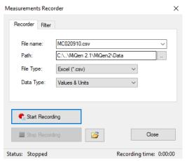
Window for setting local database recording parameters
