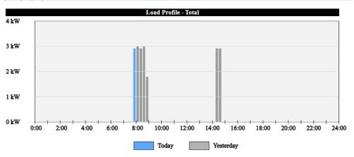
Total energy consumption in last 24 hours: 4.88 kWh Max Total power in last 24 hours: 3.00 kW Min Total power in last 24 hours: 0 W
