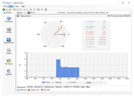
Online measurements in graphical form – phaser diagram and daily total active power consumption histogram
