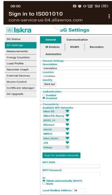
Figure 13: SG scanned available Wi-Fi networks
